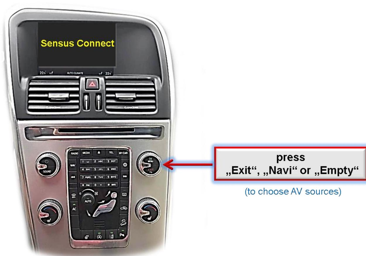
Switching the video sources can be done by a long press of the vehicle's „Exit“, „Navi“ or „Empty“ buttons.
