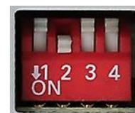
**After each Dip-switch-change a power-reset of the Can-box has to be performed!**
