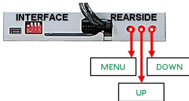
The picture settings are adjustable by the 3 push-buttons at the rear-side of the video-interface. Press the MENU button to open the OSD settings menu or to switch to the next menu item. Press UP and DOWN to change the selected value. The buttons are placed inside in the housing to avoid accidental changes during or after the installation. Picture settings must be done separately for all video inputs while the corresponding input is selected and visible on the monitor.
