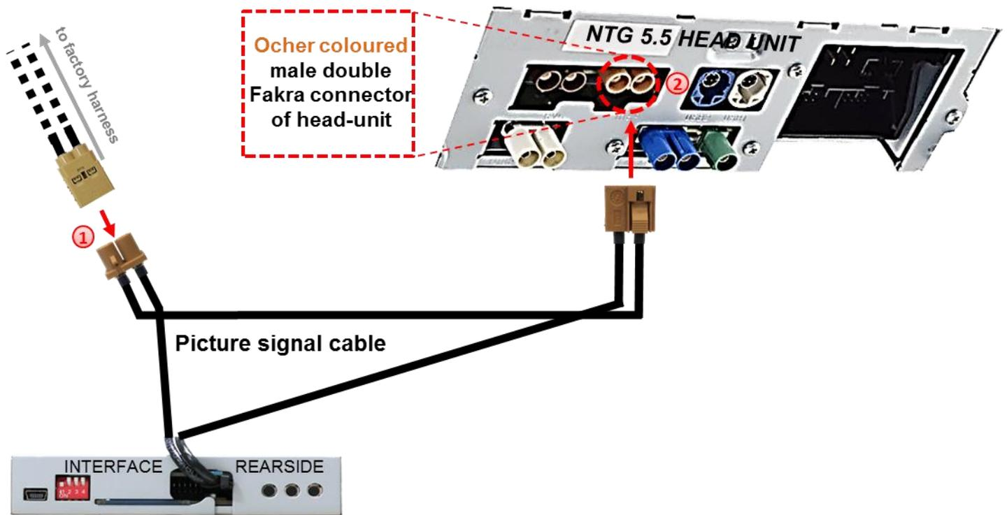
1 Disconnect the **ocher-coloured** female double Fakra connector from the rear-side of the head unit and connect it to the picture signal cable's **ocher-coloured** male double Fakra connector.
